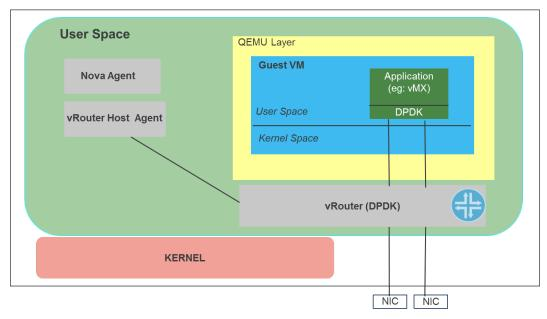
This process links with the DPDK libraries and communicates with the vRrouter host agent, which runs as a separate process. You can write an application inside of the guest VM to use the DPDK API or you can use the traditional socket API. However, for NFV applications such as vMX, which require high performance, using the DPDK API inside the VM is preferable.
