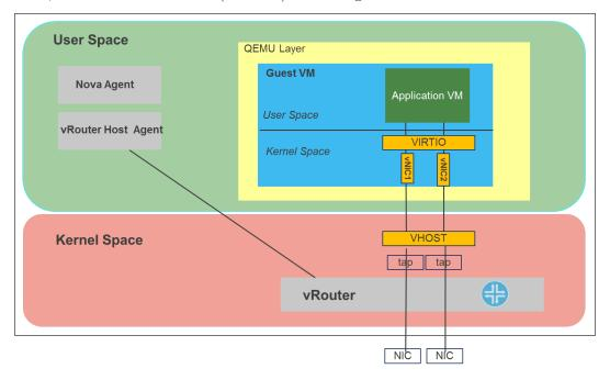
The vRouter module can fill a 10G link with TCP traffic from a virtual machine (VM) on one server to a VM on another server without making any assumptions about hardware capabilities in the server NICs. Also, to support interoperability and use a standards-based approach, vRouter does not use new protocols and encapsulations. However, in network function virtualization
