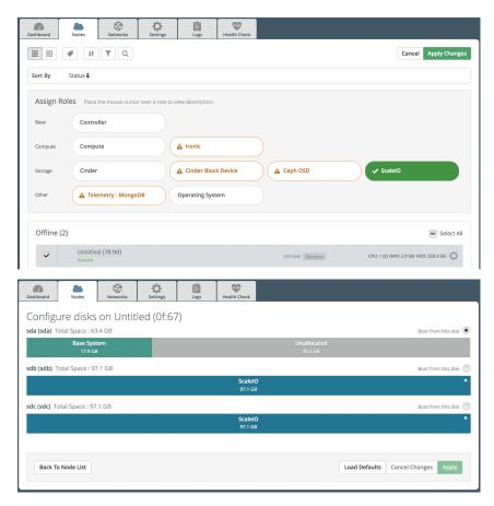
d. In case of hyper-converged deployment enabled make disks for ScaleIO SDS devices unallocated.
